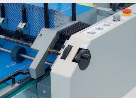
All elements for the sheet size adjustment have been centralised. The operating panel gives good accessibility to the operator.
