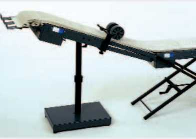
The stream delivery extension 482.105 to bring the printed material back up to table height.
